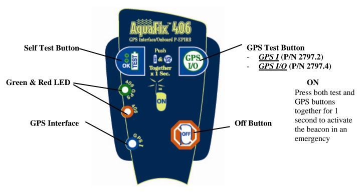
Figure 1. Key Pad Functions (P/N 2797.4 shown)
